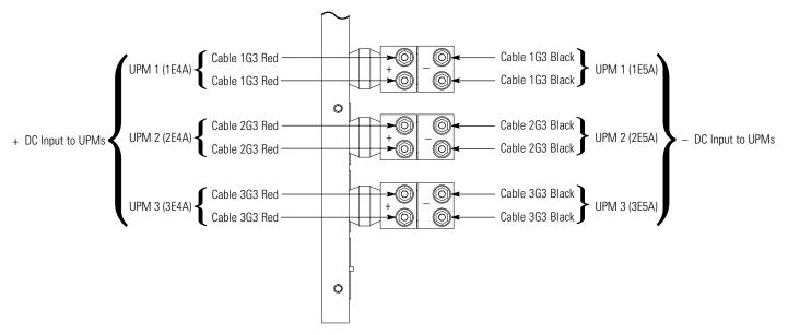
Figure 4-12. ISBM Section Battery Input Power Terminal Detail
